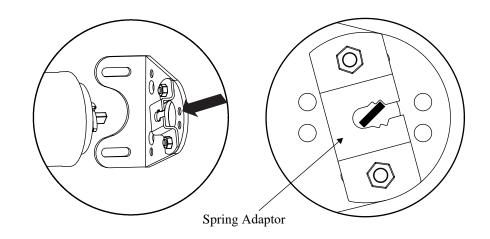
Align and insert the rectangular drive end into the spring adaptor.. When the blind is uder tension this will twist and lock into place.
