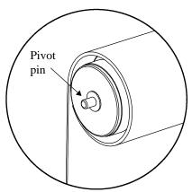
Align and locate the pivot pin into the slot in the spring adaptor.
