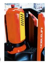
For the pallet trucks there are no hoses or pipes used in the hydraulic lifting circuit which significantly improves **reliability** and reduces the amount of potential problems related to leakages through connectors or their seals.
