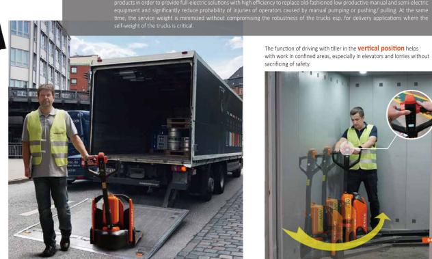
The function of driving with tiller in the **vertical position** helps with work in confined areas, especially in elevators and lorries without sacrificing of safety.
