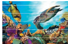
Gap/White streaks (Excessive feeding amount)
