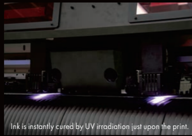
Ink is instantly cured by UV irradiation just upon the print.
