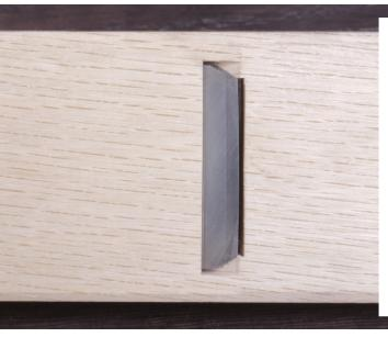
At this point, the new plane's blade is reinserted with five firm taps to establish where it is seated. This plane's blade is about 2mm short of protruding. We are aiming for the blade to protrude enough that it can just be felt with a careful thumb, but will still be hard to see when sighting down the plane.
