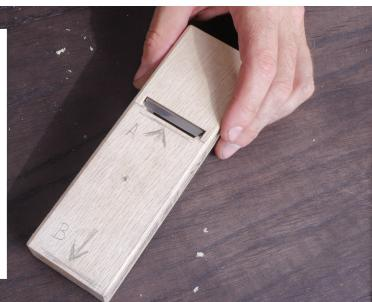
Rear of plane should be perpendicular to blade angle for hammer taps
