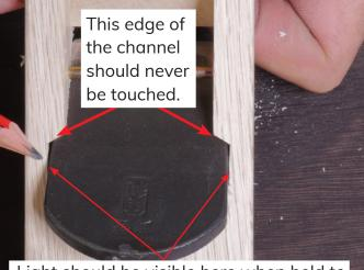
Light should be visible here when held to a light source on both sides of the plane.
