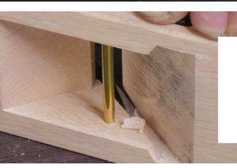
These outside edges can be carefully pared with either a 3mm chisel or a small file, depending on availability. Only a small amount of material needs to be removed - enough to ensure that the sides of the blade will not foul on the body when being seated.
