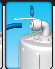
Disconnect supply line
