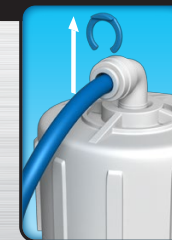
Remove retainer clip
