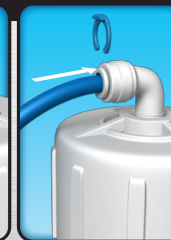
Push in & hold fitting insert
