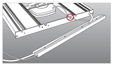
Place the fixture power cord in the lower channel and the LED cords in the upper channel. The LED cords will route through the "U" cutouts on top of the endplate..
