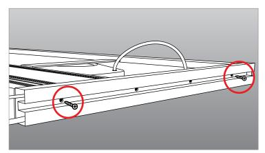
Using the metal (pointed) screws, attach the endcap using the two outer holes. These are the holes that were pre-threaded in step 4.
