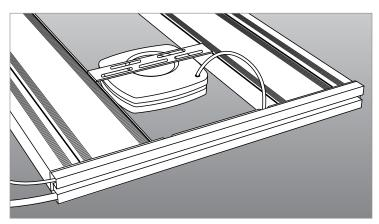
Position the décor endcap over the four open holes on the new endplate.
