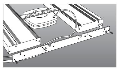
Install the new endplate using the same four screws that were removed.
