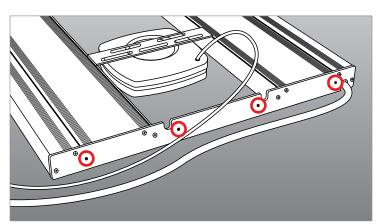
The new endplate has four additional holes. The two outer holes will accommodate the sheet metal screws. The two inner holes will use the screws with nuts.
