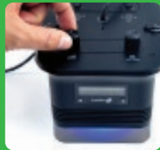
Power Knob Controls the maximum light intensity of both channels
