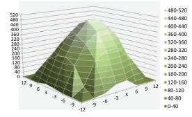
Halo Freshwater LED 110° Lens **PAR Measurements**
