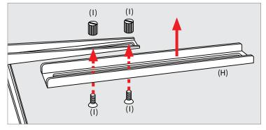
**Step 10** – Remove the screws from the end of the suspension cables and slide the screws through the channels closest to the front of the fixture. Attach each suspension cable to the screw.
