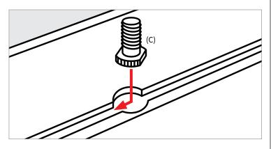
**Step 9** – Loosen the two locking screws on each pivoting bracket with a flathead screwdriver and slide the bracket to the top of the fixture. Center the fixture over the aquarium and place the bracket over the screw. Reconnect the fixture to bracket connector using the flathead screwdriver.
