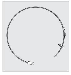
**Step 6** – Thread each suspension cable (B) through the eyelet of pivoting arm on the cantilever wall bracket (A), then through the wire screw clamp (D) to form a loop. Tighten the screws to hold the cable in place. Make sure there is plenty of slack in the cable.
