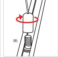
**Step 11** – Loosen the screws on the wire screw clamp with a Phillips screwdriver, and pull the cable tight. Tighten the screws and position the wire cable management slides (E) so they hold the excess cable neatly in place.
