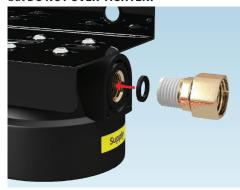
**Step 3** – Insert a 1/2" rubber washer into the side labeled **FILTERED** and then thread the Quick Connect x 1/2" MPT fitting into that side. **HAND-TIGHTEN ONLY.**
