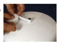
**Step 2** – Thread the Pressure Tank Valve onto the ¼" nipple on the end of the Water Storage Tank and hand tighten.
