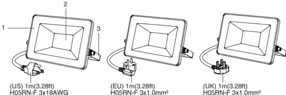
**EN** 1. Tempered Glass Lid 2. LED Light Source 3. Lamp Bracket
