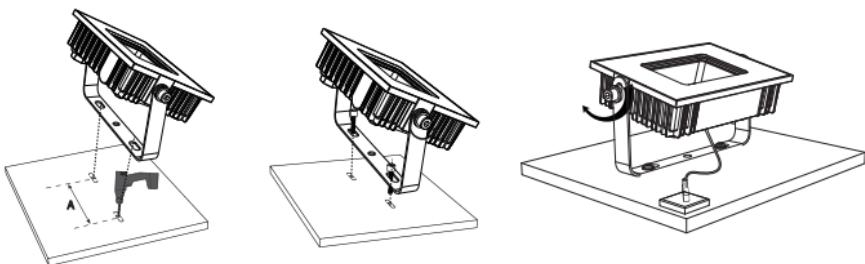
**EN** Step 1: According to the spacing (see the "A" part of the picture) of two screw bits on the LED Light bracket, drill two mounting holes.
