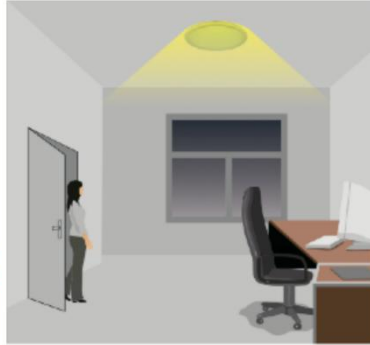
With insufficient ambient light, the sensor will switch ON the fixture when motion is detected.
