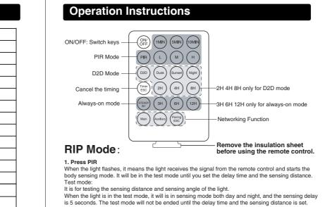
Note: Every time press RIP, the light will be in the test mode until you adjust the setting.
