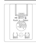
Replace the batteries of the remote control by referring to the figure on the right.
