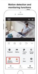
To activate the motion detection and monitoring functions, you need to turn on "Motion Detection" and "PIR" at the same time. With these functions you can receive photos and aler notifications that the camera automatically captures when detecting a motion. After setting Motion Detection and PIR, lamp can be triggered to turn on automatically if camera is in the darkness.
