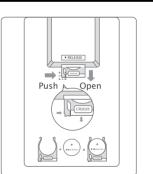
Replace the batteries of the remote control by referring to the figure on the right.
