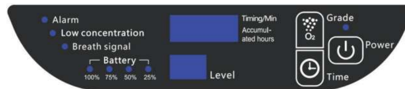
Figure 4 – Operation panel diagram
