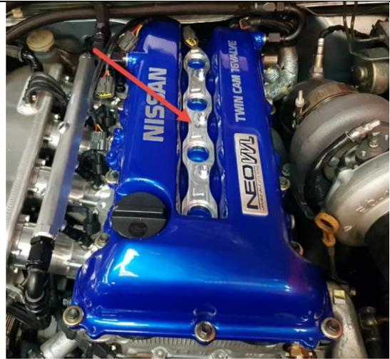
Insert the o-rings into the bottom of the billet bracket shown in the picture on the left. Remove the original coil setup and bolt your new Platinum bracket in over the original grommet and pressed steel washer, insert 1 x 55mm cap bolt with washers in the middle where indicated. (red arrow) Tighten the bolt enough to seat the bracket and slightly crush the O-rings but not enough to strip the thread in the head.
