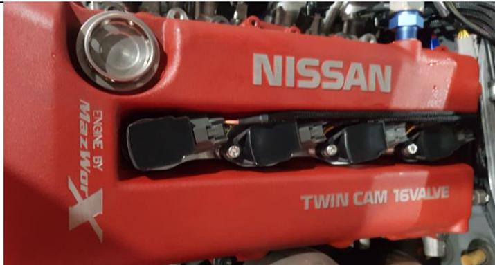
You may now insert the coils, the last 3 utilise original mounting bolts, the No 1 Cyl, will have a modified coil which is simply seated into position, and will seat itself with some downward pressure, then you may clip in your wiring loom in.
