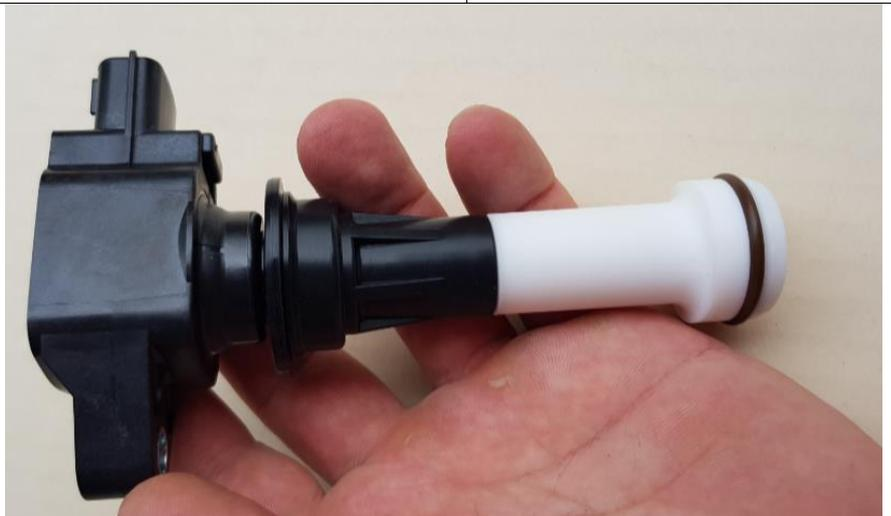
Carefully put it together ensuring the spring sits in the resistor well against the resistor
