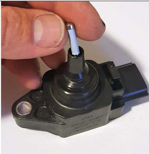
Drop the resistor into the coil head
