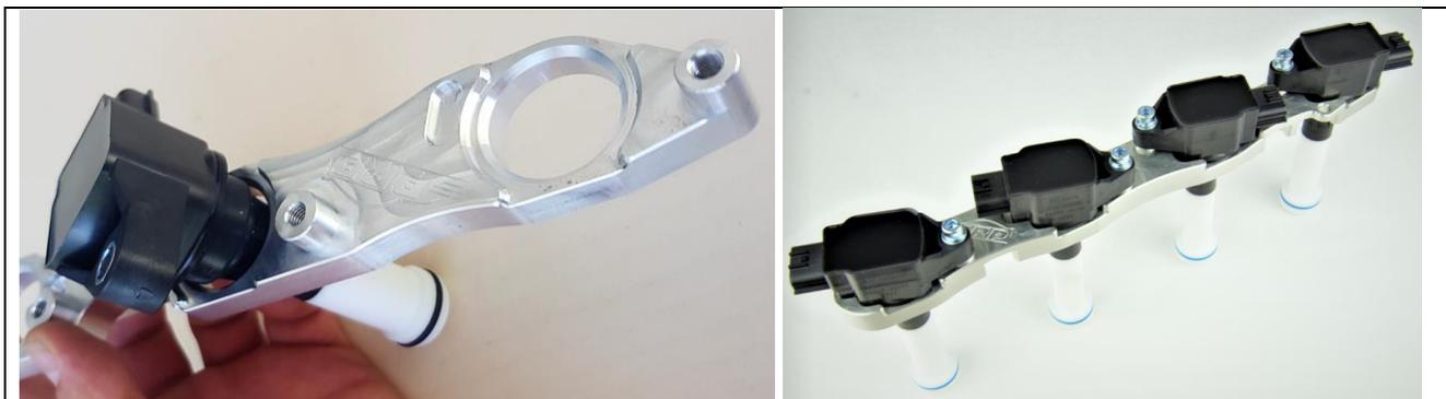
You may now insert the coils, bolt the coil down with the M6 cap bolts, spring and flat washer provided, the coil will seat itself with some downward pressure, you can bolt the bracket down first and insert the coils or put the coils together first and then install the whole kit.
