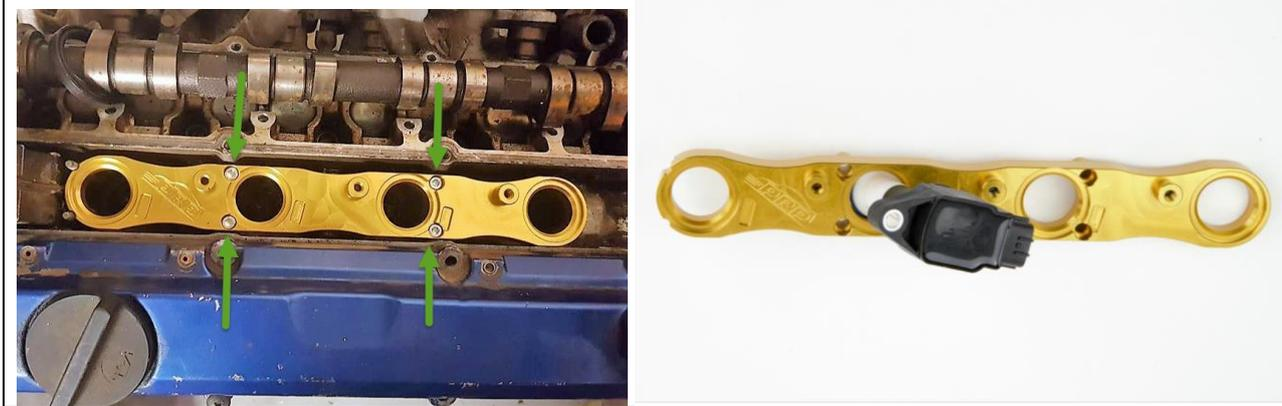
You may now insert the coils into the bracket first using the M6 bolts and washers provided, or bolt the bracket down into the head first with the smaller M5 screws provided (no washers).
