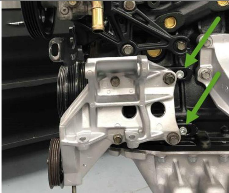
Once you are happy with your belt and pulley orientation you may tighten these rear bolts, then remove the OEM A/C Bracket and tighten the front ones, then you can put the bracket back on (don't forget the sandwiched washers)
