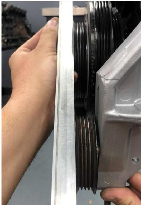
Use a straight edge to line up your pulleys for proper belt orientation, slide your bracket back and forth until its straight (ensure the idler main bolt is tight)
