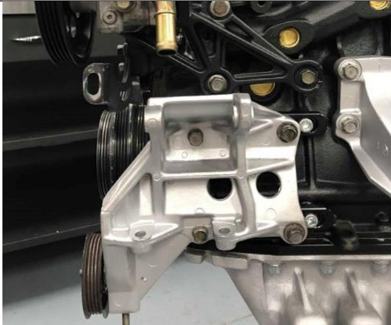
Install the OEM alloy air conditioning bracket (bolts just nipped up) with a M10 washer (supplied) between the OEM bracket and your PRP black brackets, Remember the Black brackets are on lose so the whole assembly should be free to slide back and forth with a bit of effort.
