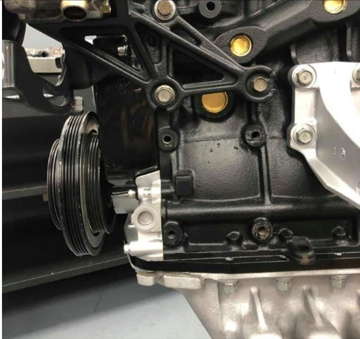
Remove the air conditioning compressor and OEM bracket
