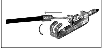
Pull the upper tension Connector backward and slide the wire through the slot on the bracket.
