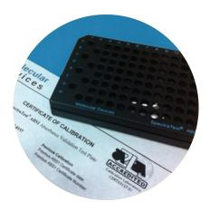
Validation plates for optical performance. SpectraTest Validation Test Plates for absorbance and fluorescence intensity provide a complete traceable solution for validating optical performance of the SpectraMax M2 reader, automatically.
