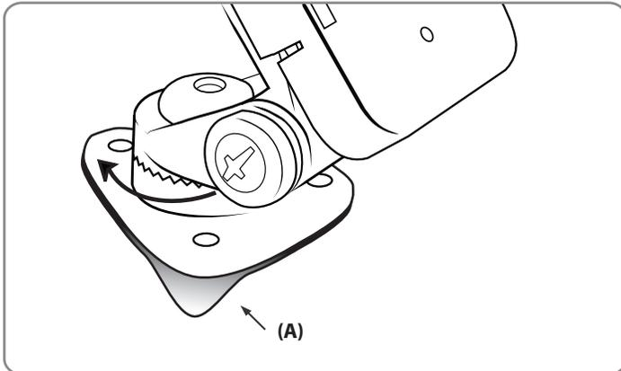
Step 2. Remove the adhesive backing (A) under the triangular pedestal and firmly press into place.
