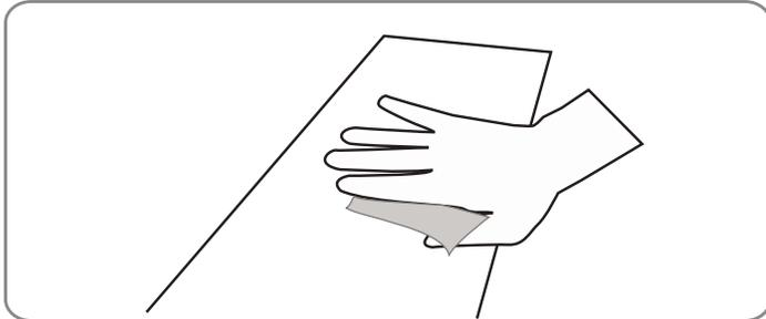
Step 1. Find a safe location on the dash or console to mount the pedestal. Make sure the area is clean and dry. Use the included alcohol pad to clean the mounting surface.
