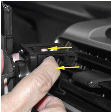
1 Fully retract both spring vent clips with fingers.
