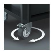
The two swivel castors are equipped with a double stop: The locked castor reliably prevents it from rolling away, the locked spindle carrier prevents the castors from turning unintentionally, e.g. on sloped surfaces. The oil- and acid-resistant elastic wheels ensure smooth running. A protective ring prevents the ingress of dirt and threads.
