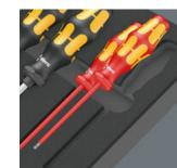
After removing the tool the light grey second foam becomes visible and therefore missing tools are quickly identified.
