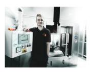
The individual testing at 10,000 volts, in accordance with IEC 60900, ensures safe working with loads up to 1,000 volts.
