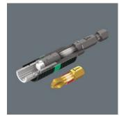
The optimally coordinated features of the torsion zones on the bit and holder permit a phased yield when under strain. The two-phase system prevents premature wear. Moreover, a long tool service life is also ensured by the hardness of the bits that matches the respective application.
