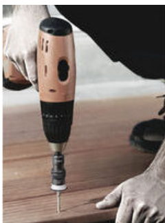
Bit holder for evenly flush countersunk screws in patio construction
