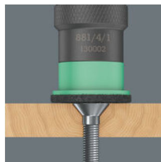
The 881/4/1 bit holder allows for evenly flush countersinking of screws in decking when building patios. The screw depth can be adjusted as required. This prevents screws from being countersunk too deep.
