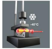
Impact strength tested at -40°C, guaranteeing safety even under extreme conditions.
