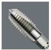
cutting Tap bits Application: Cutting threads1/4" drive suitable for holders as per DIN (ISO 3126-D 6.3 1173)Hexagon shaft for very high torque transferFinely adjusted material elasticity for long service lifeExcellent centring propertiesStraightforward cuttingPerfect chip removalLow jamming riskPrecise return controlHigh corrosion protection
