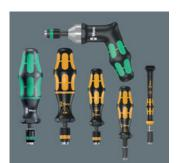
Wera torque screwdrivers. With a factory pre-set torque value set to the smallest scale value. For all applications, where the same constant torque and repeat accuracy are required. The torque can be changed with an extra tool within the measuring range (recalibration kit can be ordered with the code number 05137003001). Afterwards you can check the set value using an off-the-shelf torque tester.
