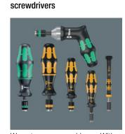
Wera torque screwdrivers. With a factory pre-set torque value set to the smallest scale value. For all applications, where the same constant torque and repeat accuracy are required. The torque can be changed with an extra tool within the measuring range (re-calibration kit can be ordered with the code number 05137003001). Afterwards you can check the set value using an off-the-shelf torque tester.
