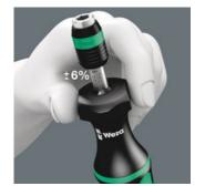
Measurement accuracy is  $\pm$  6 % (article 1430:  $\pm$  10 %) in accordance with the standard DIN EN ISO 6789. Distinctly audible and noticeable excess-load signal when the pre-set torque is reached.
