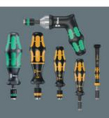
Wera torque screwdrivers. With a factory pre-set torque value set to the smallest scale value. For all applications, where the same constant torque and repeat accuracy are required. The torque can be changed with an extra tool within the measuring range (re-calibration kit can be ordered with the code number 05137001001). Afterwards you can check the set value using an off-the-shelf torque tester.
