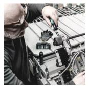
Many screws - particularly in assembly and maintenance applications - have to be tightened with controlled torque to ensure the dependability of the screw connection and/or to avoid damage to the screw or work piece. Wera's adjustable torque screwdrivers are the ideal tool for this. They feature a torque range of 0.3 Nm to 8.8 Nm, two different handles, measurement accuracy of  $\pm$  6 % and Rapidaptor technology for rapid bit change.
