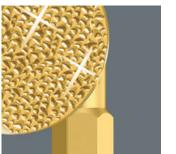
The minute diamond particles applied to the tip of the tool literally "bite" into the screw and ensure an exact, anti-slip fit in the head of the screw. This secure fit protects the screw. The cam-out forces which compel the user to apply greater pressure to the screw are considerably reduced.
