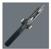
The 4-in-1 bit 9506 can be used to operate four sizes of hexagonal socket screws (3.0; 4.0; 5.0; 6.0). In order to use the larger profile, continuously press against the spring tension while screwdriving so that the smaller profile is countersunk and the larger profile can be used.
