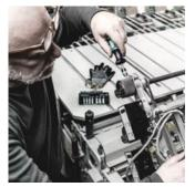
Many screws - particularly in maintenance assembly and applications - have to be tightened with controlled torque to ensure the dependability of the screw connection and/or to avoid damage to the screw or work piece. Wera's adjustable torque screwdrivers are the ideal tool for this. They feature a torque range of 0.3 Nm to 8.8 Nm, two different handles, measurement accuracy of  $\pm$  6 % and Rapidaptor technology for rapid bit change.
