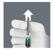
Simply push the sleeve forward to change the bit. The spring mechanism lifts the bit off the magnet and unlocks the tool. The bit can be easily removed. The rapid-out function makes it easy to remove even the smallest bits without extra tools.
