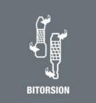
Peak forces that occur in power tool applications often result in premature wear of bits or damage to the screw head. This usually occurs during initial power-up and the when the screw comes to a standstill. Screwdriving could become more productive and safer if these peak loads could be minimised. The Wera BiTorsion system prevents premature wear. The service life of the tool is extended and the productivity of applications power tool significantly increased.
