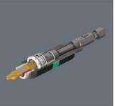
The effectiveness of the BiTorsion system comes from a combination of two shock-absorbing spring elements. Both, bits as well as holders have a cushioning torsion zone that diverts the kinetic energy away from the drive tip during peak loads.
