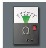
The electric surface resistance of the Wera ESD material is  $\leq$  10<sup>9</sup> ohm. This securely protects components against electrostatic energy and associated damage.
