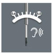
Distinctly audible and noticeable excess-load signal when the preset torque is reached.
