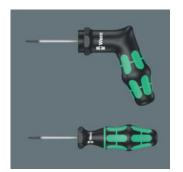
Wera torque-indicators have been factory pre-set to values recommended by leading carbide manufacturers. These tightening values relate specifically to the size of the TORX®, TORX PLUS® or hexagon socket screw. Torque indicators ensure safe and loosening easy of screw connections. Precision :  $\pm~10~\%$
