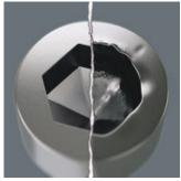
Hexagon socket screws are a problem, because the contact surfaces that transfer the force of the tool to the screw are very narrow. The consequence: the head of the screw can be damaged, usually rounding out the recess. Hex-Plus tools have larger contact surfaces to prevent this, driving from the flats of the recess, rather than the corners. Good to know: Hex-Plus tools fit into every standard hexagon socket screw!
