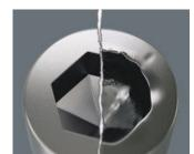
Hexagon screws can endure a problem because the contact surfaces delivering the power from the conventional tool, is transferred to the screw via very small surface areas. The consequence: the screw can become damaged (rounding out). Hex-Plus tools have a greater contact surface that prevents this from happening! At the same time, as much as 20 % more torque can be applied. Good to know: Hex-Plus tools fit into every standard hexagon socket screw!
